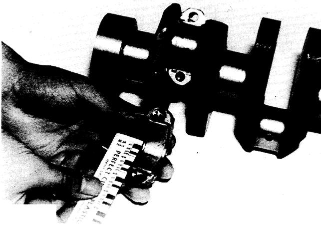
Crank pin measuring points
